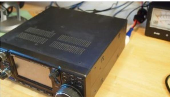
Remove all 10 screws on the top cover and 2 screws from each side.
