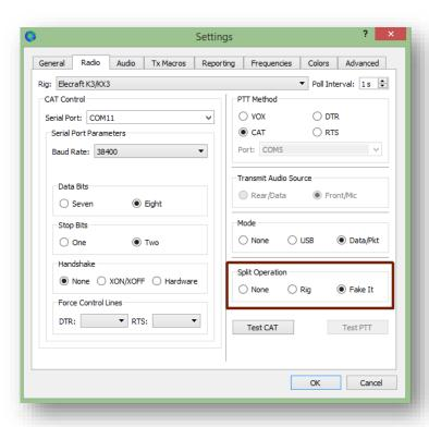
QSY commands at the start and end of every over. The "Rig" setting attempts to use the split function built-in to modern radios by receiving on VFO A and transmitting on VFO B ... but unfortunately WSJT-X v1.8.0 does not check the radio nor re-send the split and mode commands with every over. With the "Rig" setting, if for some reason split gets disabled on the rig itself (e.g. for a simpley OSO on another mode or hand), he sure
